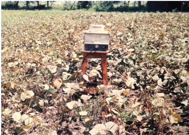
Fig.1. Volumetric Tilak Air Sampler operating in bean field for air monitoring of urediospores of Uromyces rust during kharif season of 2012 at the outskirts of Pune city.
